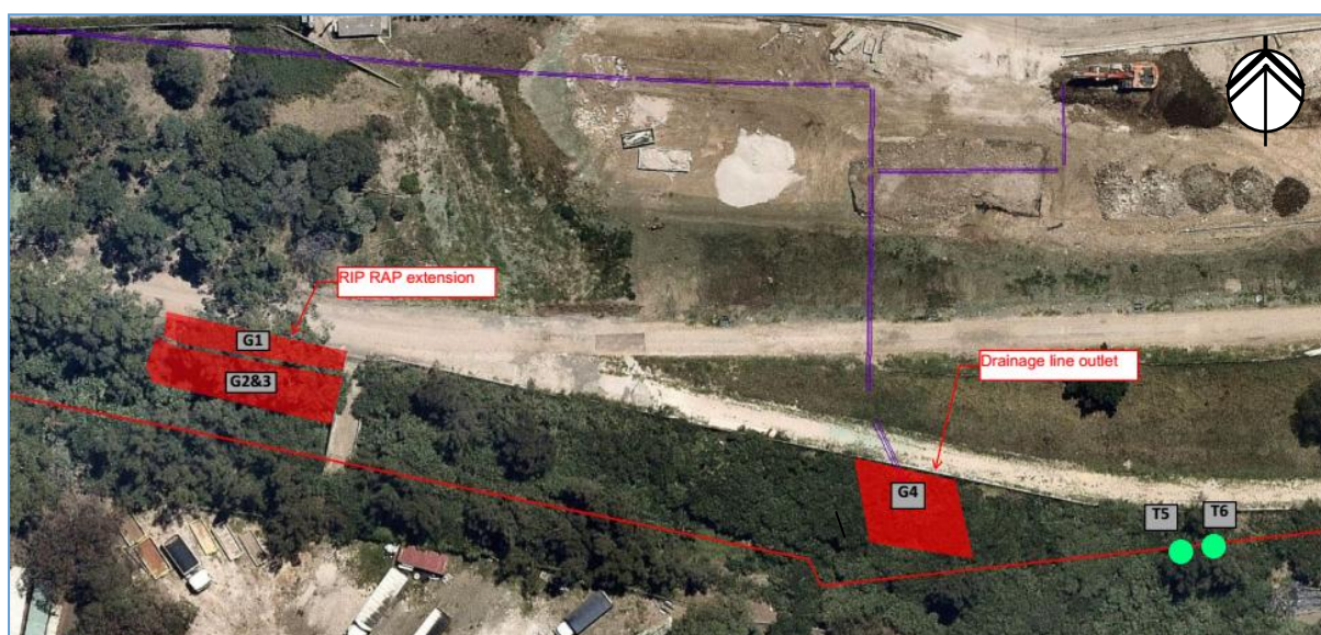
Figure 2 – Marked up Aerial. Red blocked areas indicate trees/groups proposed for removal. Green dots indicate trees to be retained. Red line indicates permanent boundary.
