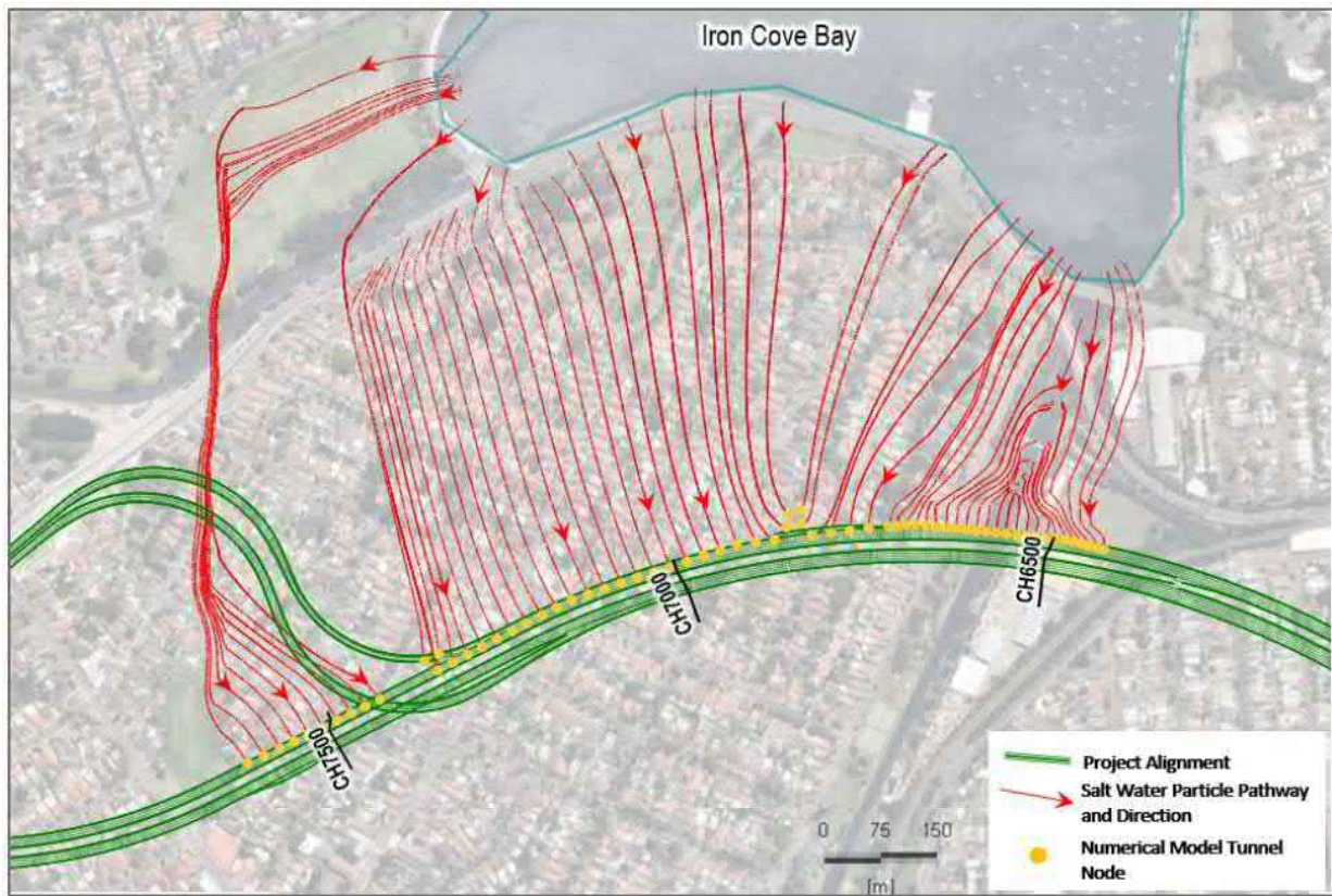
Figure 4-2 Predicted Saltwater Particle Pathways for Mainline Carriageway Tunnels at 100 Years after Excavation
