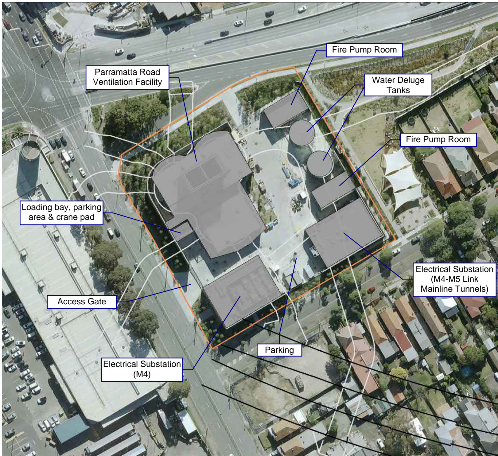
Figure 2-3: Parramatta Road Ventilation Facility
