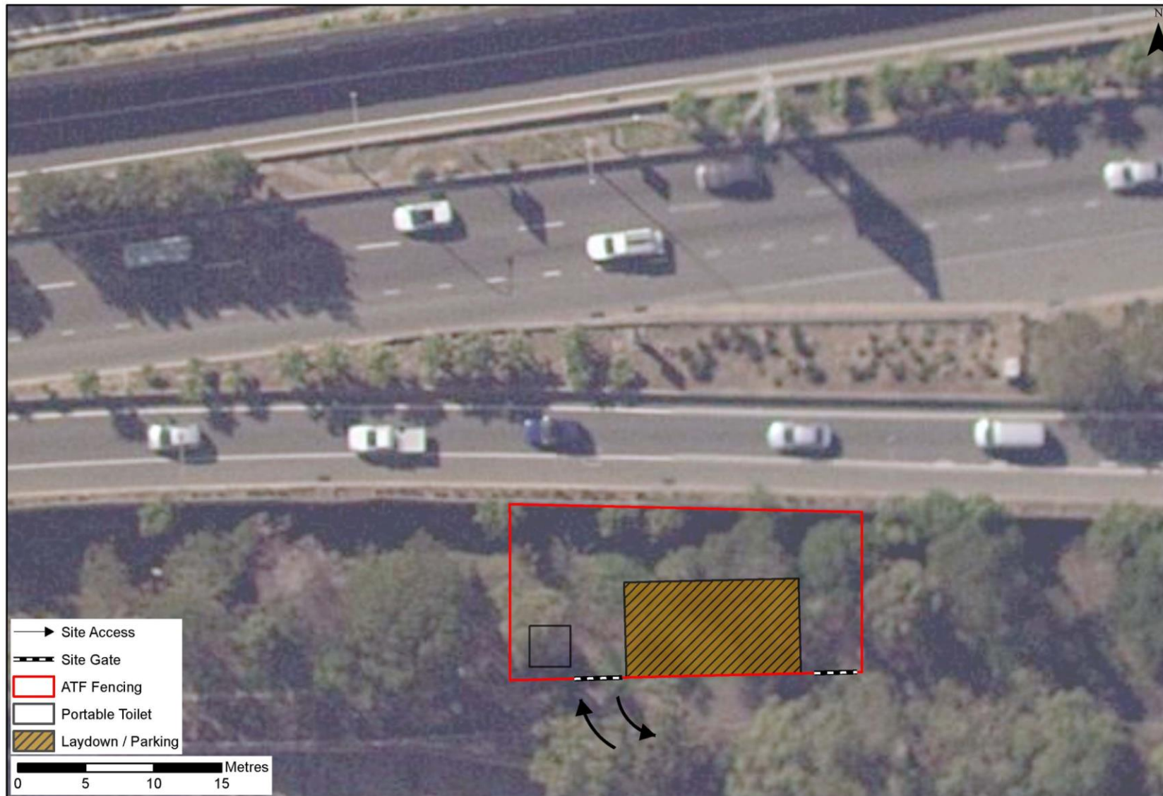
Figure 4: Bexley Interchange site layout and access route
