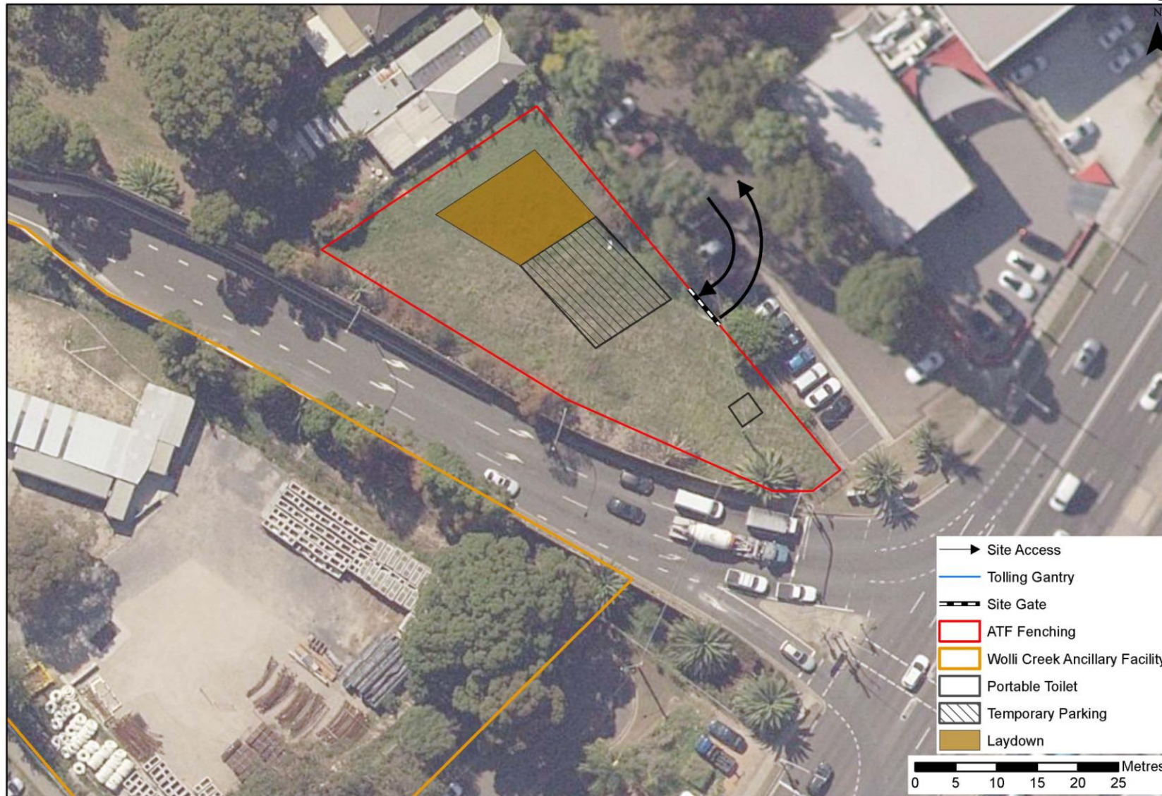
Figure 5: Princes Highway Interchange site layout
