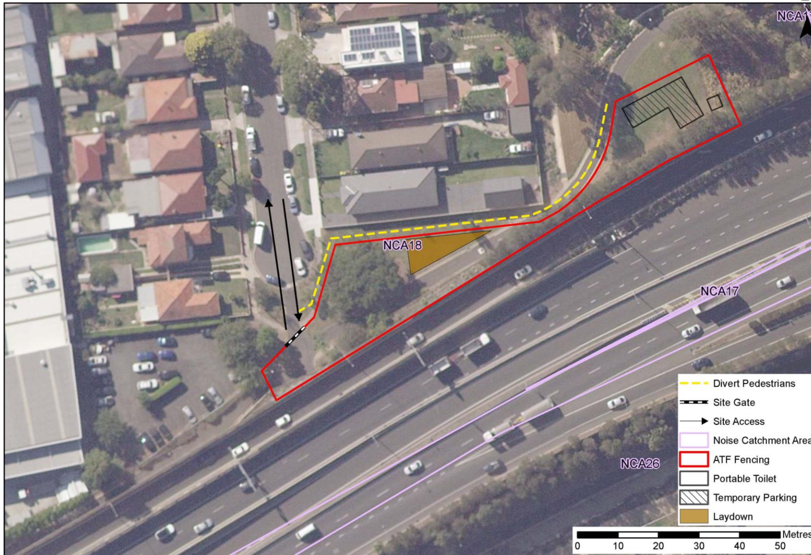
Figure 2: Kingsgrove Interchange site compound layout
