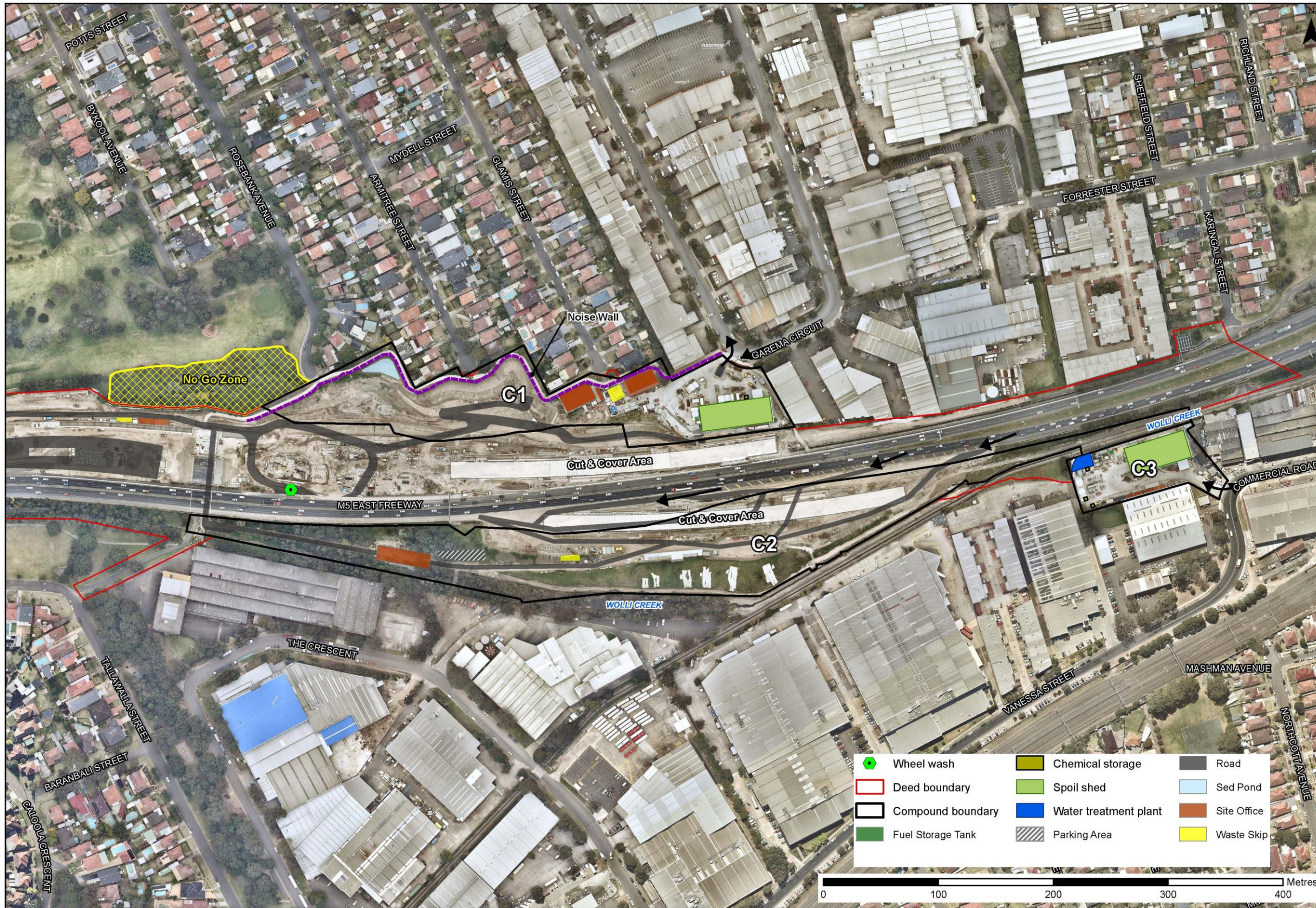
Figure 12: Kingsgrove Construction Compounds (C1, C2 & C3)
