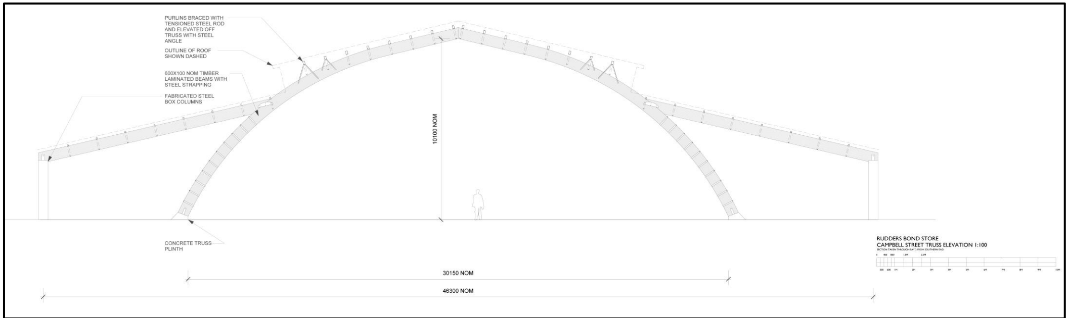
Figure 4. Section plan of laminated timber arch (Source: The Archivist , Drawing No RBS_MD-03, Issue 21.07.16).
