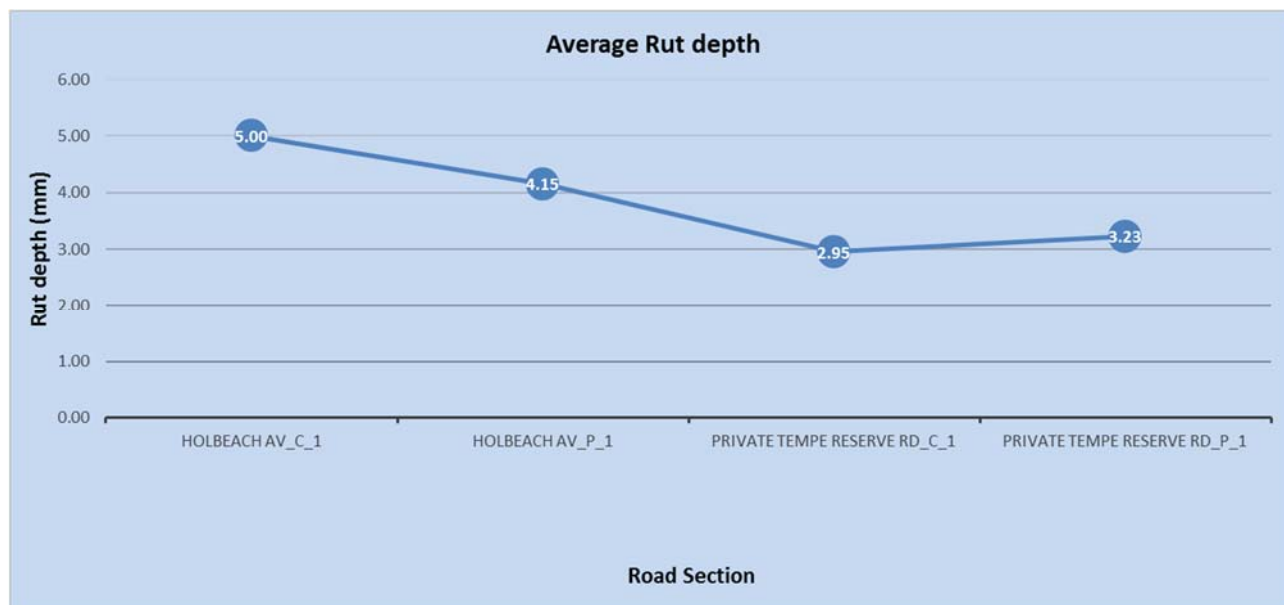
Figure 3.1: Average condition-Rut depth-Inner West Council
